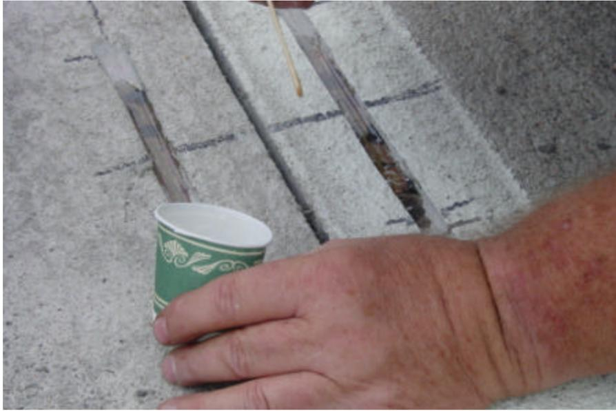
**Figure 23. Attaching Strain Gages using Fast-Setting Epoxy**
