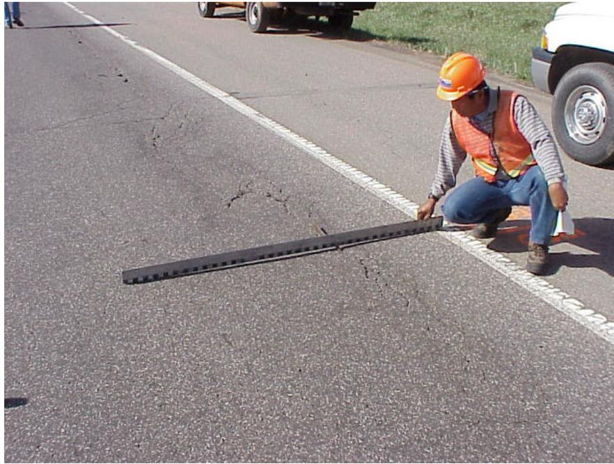
**FIGURE 4. RUTTING MEASUREMENT ON EXISTING ASPHALT PAVEMENT**
