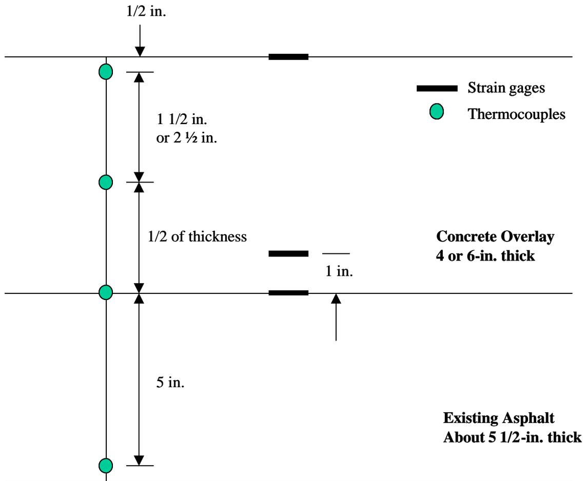
Figure 9 Typical Test Slab Layout -- Section View
