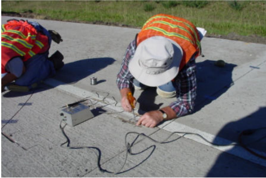
**Figure 25. Soldering Leads to Installed Surface Gages**
