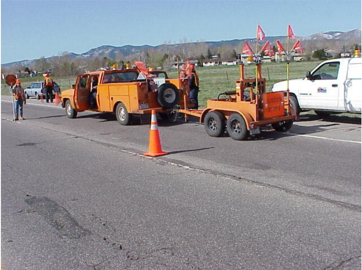
**Figure 6. FWD Testing on the Existing Asphalt Pavement**
