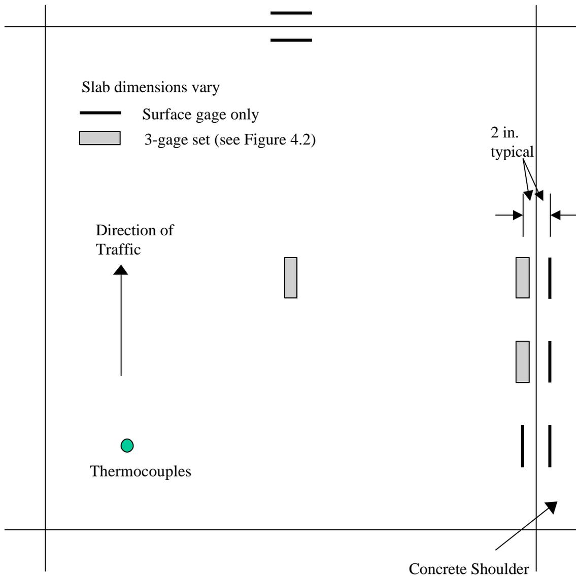
**Figure 8 Typical Test Slab Strain Gage Layout -- Plan View**
