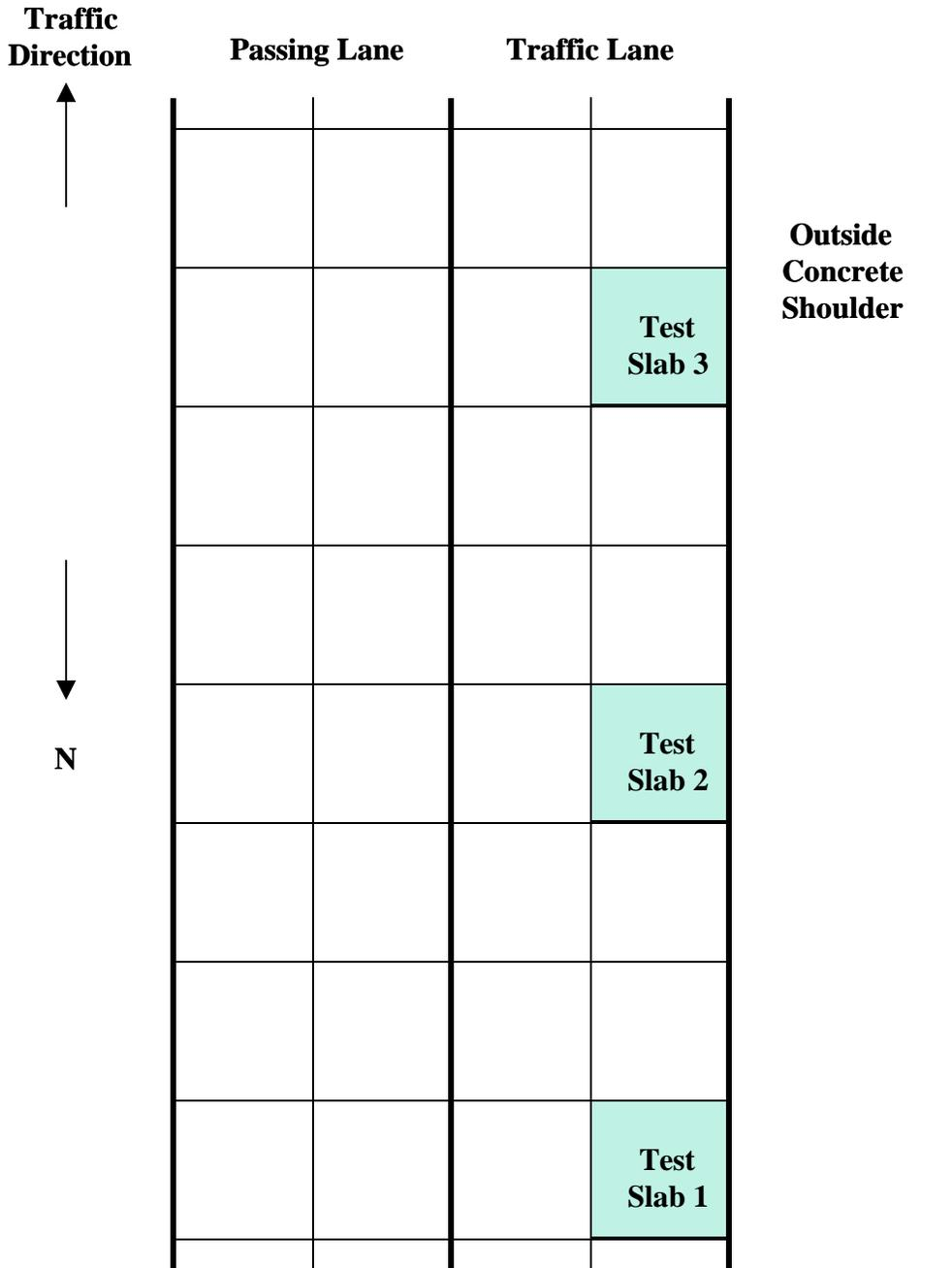
**Figure 7. Typical Layout of Test Slabs Within Each Test Section**
