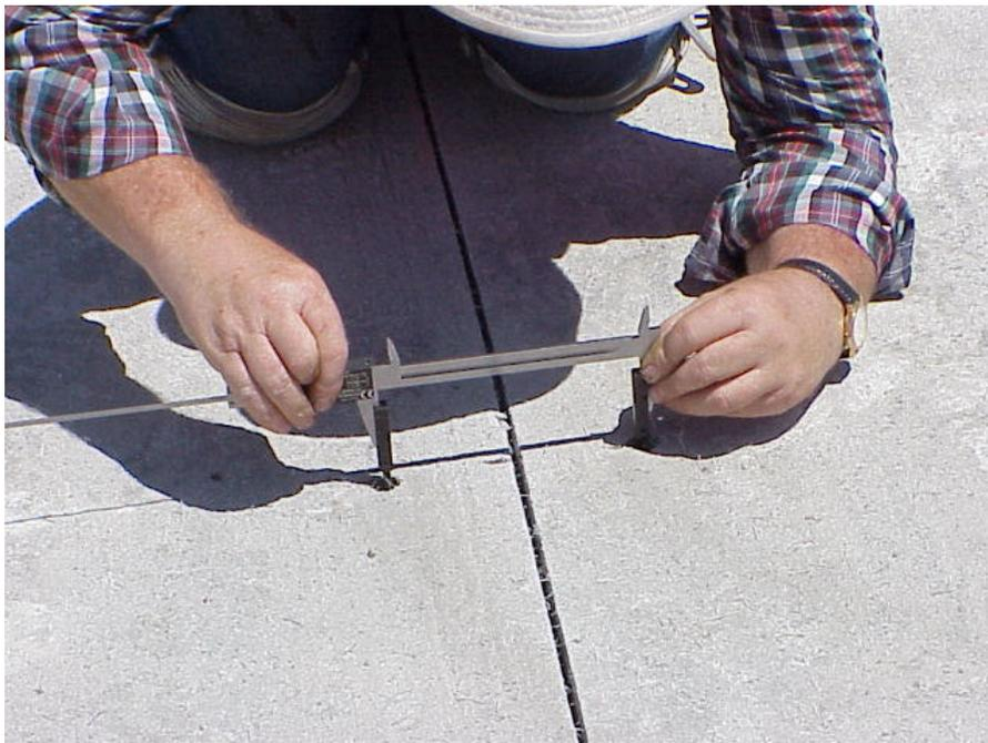
**FIGURE 20 WHITMORE PLUGS AND INITIAL MEASUREMENT**
