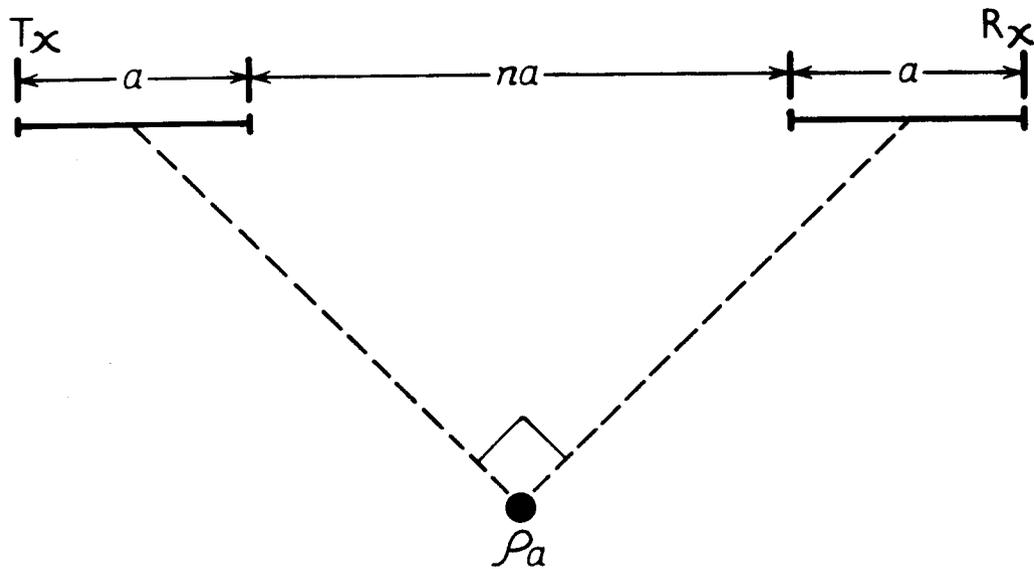
Figure 18. Data plotting scheme for dipole-dipole array (from Combs, 1980).
