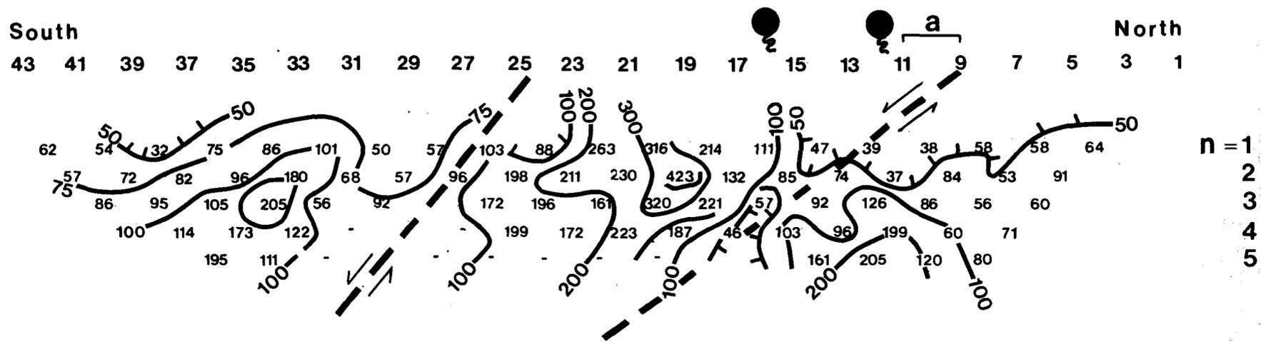
LINE C - This dipole-dipole line trends north-south and is parallel and adjacent to the narrow gauge railroad (Fig. 7). Two low resistive zones exist between stations 9 and 14 by the Big and Little Mound Springs and between stations 25 and 30. Both of these low resistive zones are marked by tufa mounds. These low resistive zones may indicate possible faulting that show good strike alignment with the other two parallel lines. Table 5 (Appendix E) tabulates the resistivity calculations for line C.
