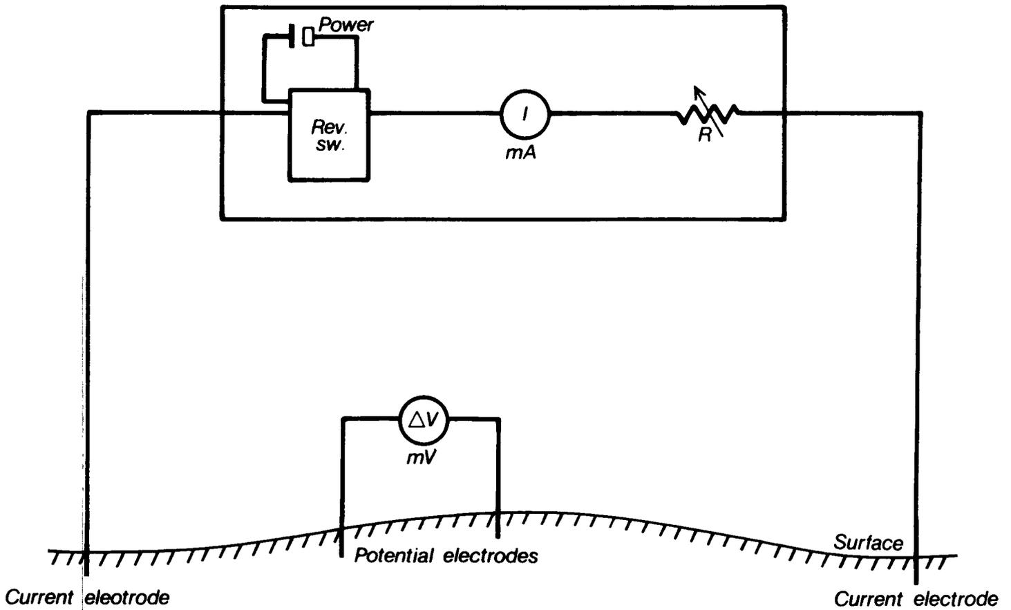
Figure 14. Schematic diagram for resistivity.
