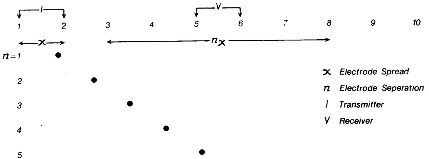
Figure 19. Typical dipole-dipole array (from Combs, 1980).
