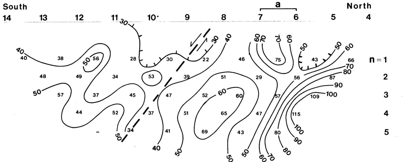
LINE D - This dipole-dipole resistivity line reflects a low resistive zone in the proximity of stations 8, 9, and 10 with the resistivity increasing to the north as the bedrock changed from alluvium to limestone (Fig. 7). The similarities that exist between line D and line A are due to a low resistivity zone at their intersection. The resistive low at Station 5 is probably due to seepage near the surface. Table 6 (Appendix E) tabulates the resistivity calculations for line D.
