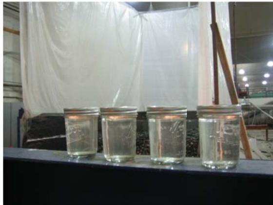
Figure 28. Water samples collected after 5min, 10 min, 15 min, and 30 min from the start of runoff.
