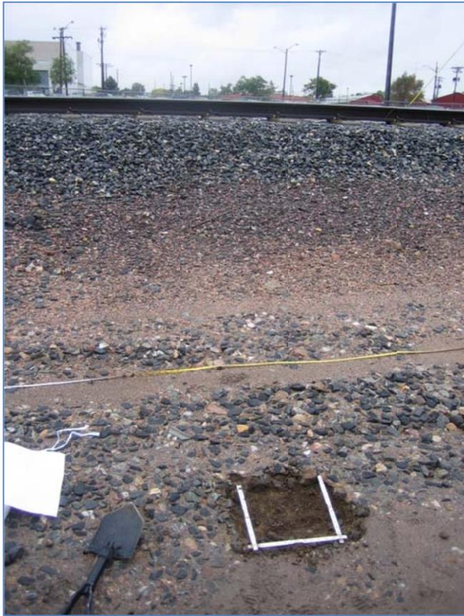
Figure 15. Soil sampling at the toe of ballasted tracks near Broadway Light Rail Station, east of I-25.
