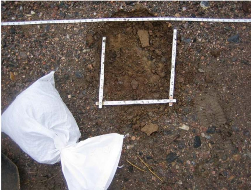
Figure 17. Soil sampling at the toe of ballasted tracks near Broadway Light Rail Station, east of I-25.
