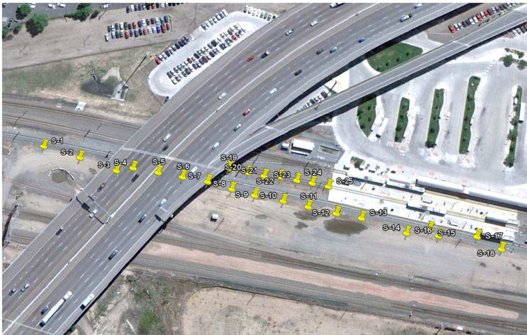
Figure 10. Soil sampling locations near RTD's Broadway Light Rail Station.
