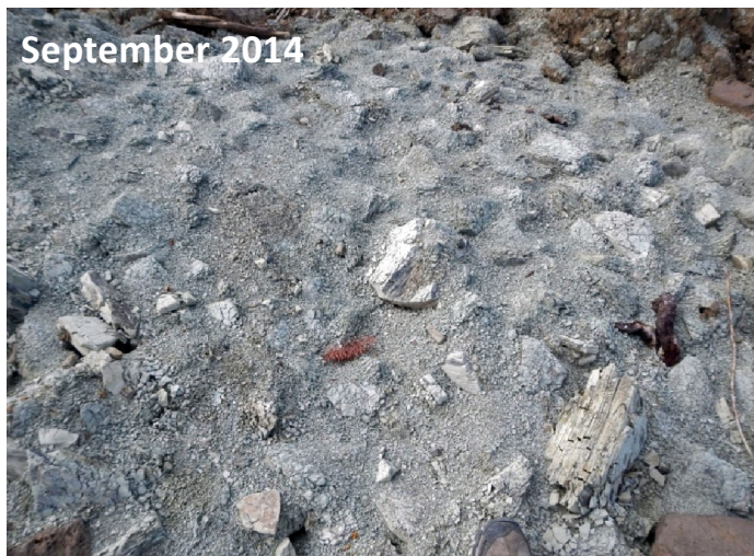
Figure 16. Rapid slaking of Green River Formation claystone and marlstone clasts in the WSCL debris field. Note surface staining of clasts and progression, clockwise from upper left, of rock disintegration in less than 4 months.
