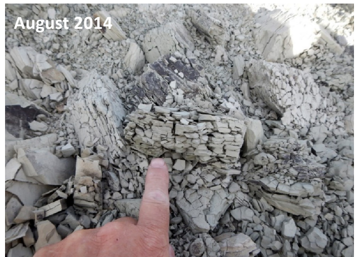
Figure 16. Rapid slaking of Green River Formation claystone and marlstone clasts in the WSCL debris field. Note surface staining of clasts and progression, clockwise from upper left, of rock disintegration in less than 4 months.
