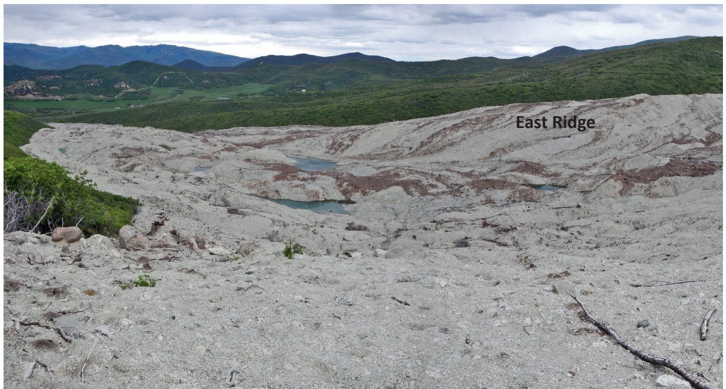
Figure 21. A year after the WSCL, large ponds formed on the hummocky late-surge rock/debris avalanche deposits. View is to the northeast from the West Ridge at the same location of Figure 11g. Note finer-grained debris field in foreground compared to Figure 11(g), as a result of year-long slaking of Green River Formation clasts. Photo date: June 5, 2015. Photo location is shown on Figure 9 map.
