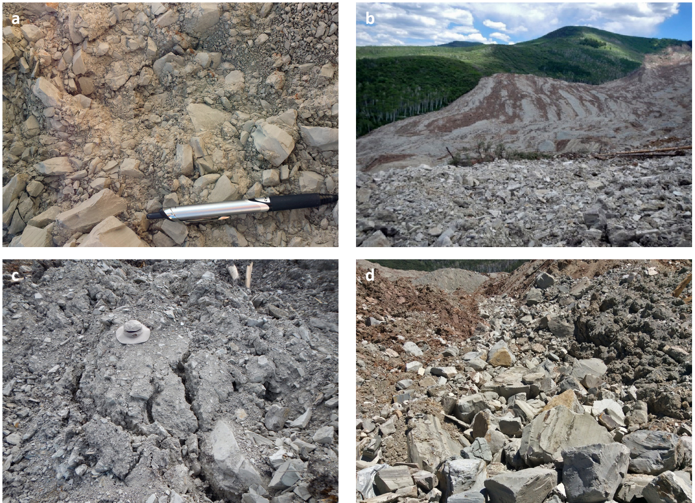
Figure 10. Rock avalanche debris locations: (a) typical matrix of avalanche deposit. Note pen for scale; (b) typical rocky debris field on west ridgeline. Note red-soil zebra-stripes related to spread of surficial soils on east flank; (c) subsidence fissures in deposit; (d) bouldery segregation within late-surge hummocky rock-debris flow; (e) debris on rise of west ridge spill over, red circle encloses person for scale; (f) east edge of debris field near toe. Photos taken summer of 2014. Photo locations are shown on Figure 9 map.
